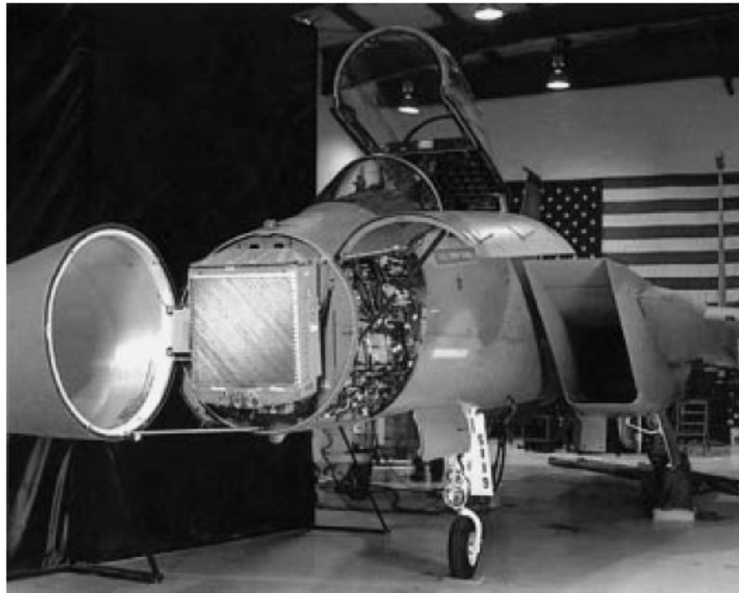
18 operational F-15Cs have been refitted with Raytheon's APG-63(v)2 AESA.
