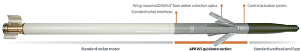
Figure 4.10. APKWS all-up round major components. Source: [71].
