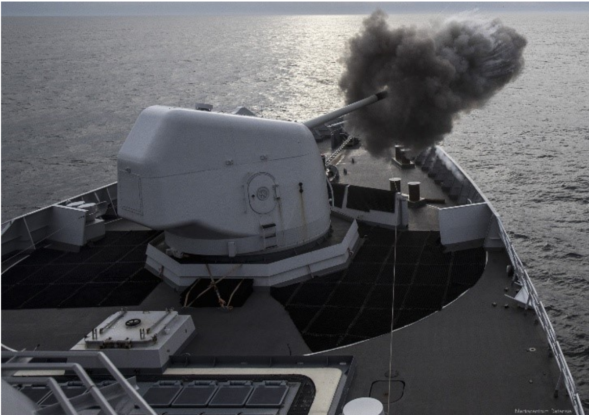
Figure 4.4. Mk-45 Mod 2 firing from a Royal Netherlands Navy De Zeven Provinciën-class frigate. Source: [64].
