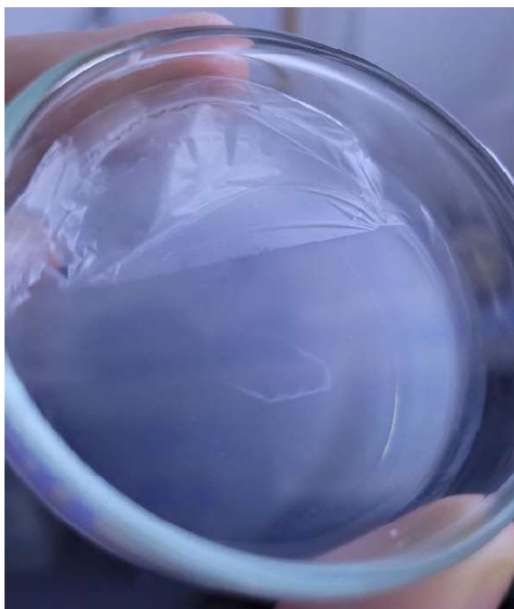
Figure 47: Polymeric film formed on a glass plate after natural evaporation of the solvent.
