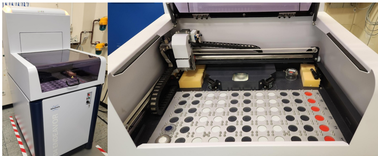
Figure 14 – D4 Endeavour Powder X-Ray Diffractometer from Bruker AXS GmbH, used for the P-XRD analysis of the \text{UO}_2 pellets.
