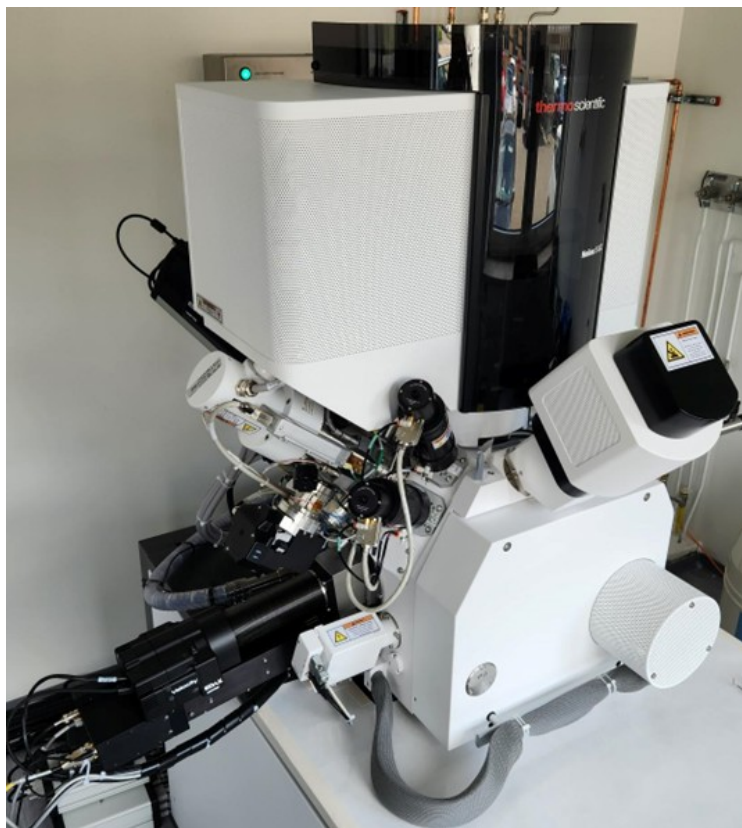
Figure 18 – Helios 5UC Dual Beam (Thermoscientific, Netherlands) for focused ion beam scanning electron microscopy (FIB-SEM) for materials science.
