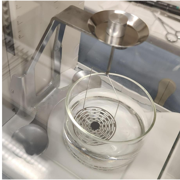
Figure 19 – Archimedes setup with suspended scale in water on a Mettler-Toledo XP205-DeltaRange Scale with a Mettler-Toledo Density Accessory Kit
