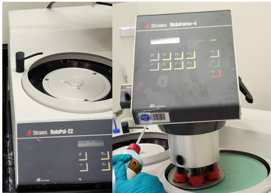
Figure 15 – Struers RotoPol-22 and RotoForce-4 setup for machine polishing.
